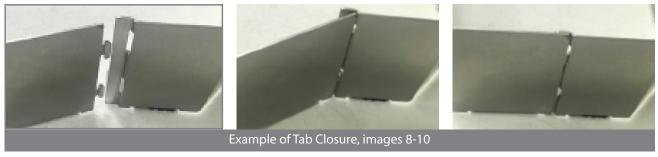
b. Swing halves together and connect angled tabs into slots.
